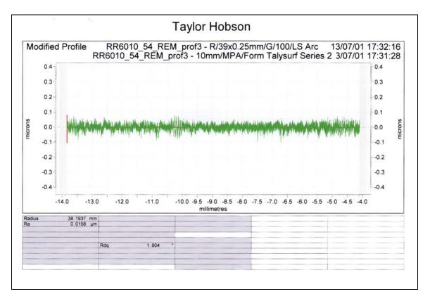
Fig 5. Profilometer trace of disc surface superfinished with plastic media.
