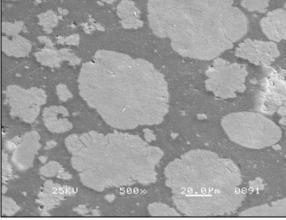
Fig 2. SEM images at 500X of the ceramic (top) and plastic (bottom) media used to superfinish the surface of the specimens.
