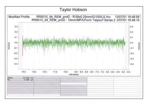
Fig 4. Profilometer trace of disc surface superfinished with ceramic media.
