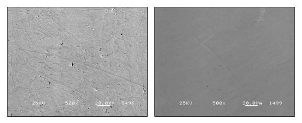
Fig 3. SEM images at 500X of surfaces superfinished with ceramic (left) and plastic (right) media.
