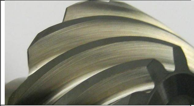
Initial ground surface of drive side (concave) of pinion.
