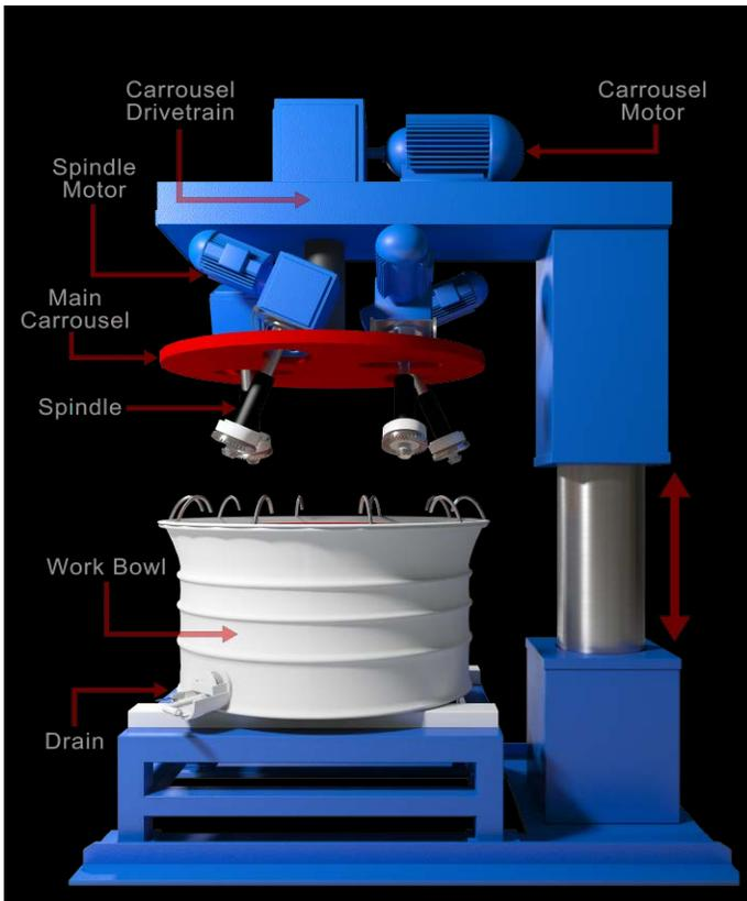
Figure 3. 3D image of the drag finisher showing the component parts.
