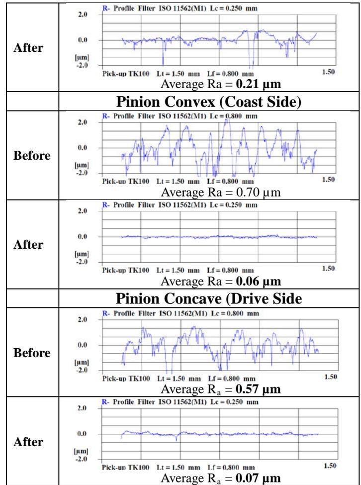
Table 3. Typical; before and after surface traces of the concave and convex sides of the ring gears and pinions after isotropic superfinishing for only 4.0 minutes.
