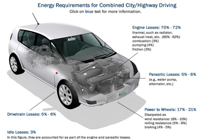
**Figure 1iii.** Shows that 5.6% of a passenger car's fuel is wasted on friction and slippage in the drive train.
