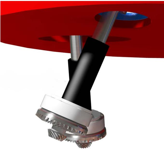
Figure 7. The spindle is attached to the drag finisher with the ring gear and pinion gear held by the magnetic force to the plastic fixture.
