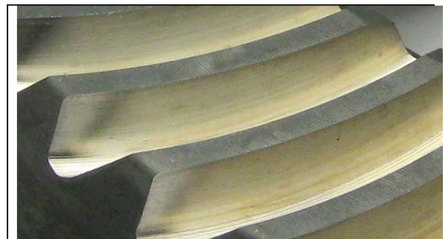
Initial ground surface of drive side (convex) of ring gear.
