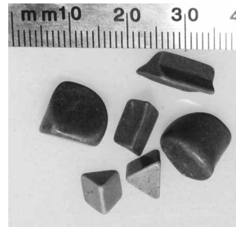
Figure 5: Sample of high density, non-abrasive ceramic media.
