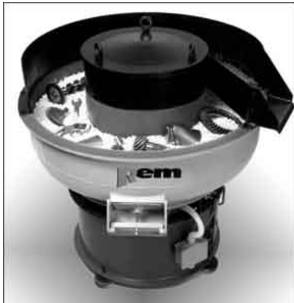
Figure 3: A 10 cubic foot vibratory bowl loaded with assorted commercial parts.
