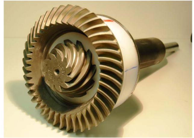
Figure 2. A matched ring and pinion gearset fixtured ready for attachment to the spindle of the drag finisher machine.
