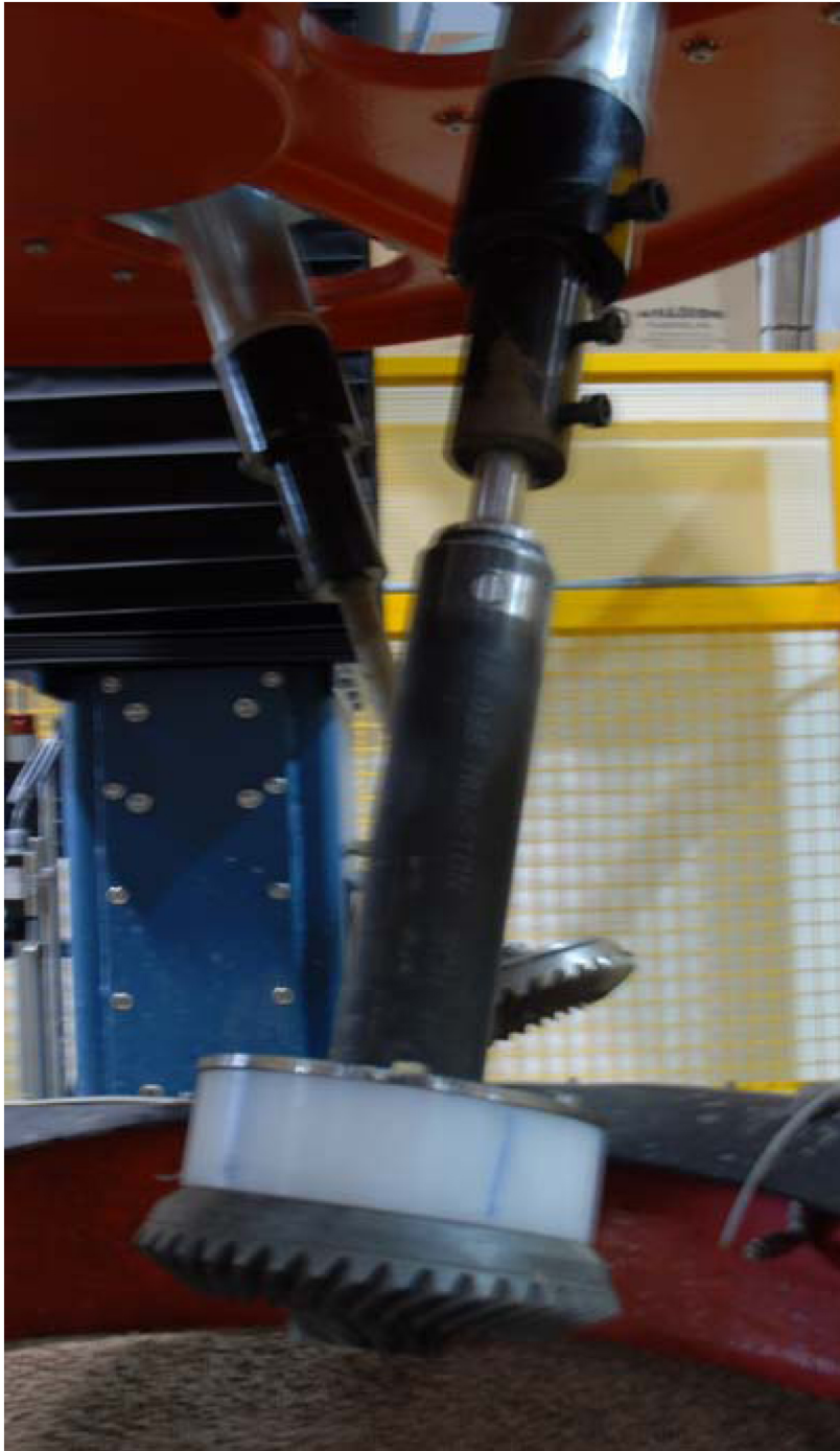
Figure 3. Picture of the Drag Finisher with one fixture holding a ring and pinion gearset attached.
