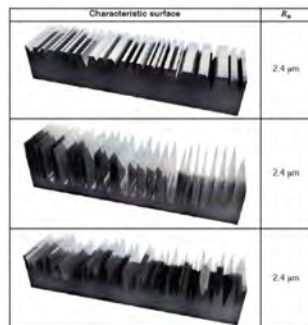
Figure 1: Examples of “equal” Ra measurements on obviously dissimilar surfaces (photo courtesy of Hommelwerke GmbH)
