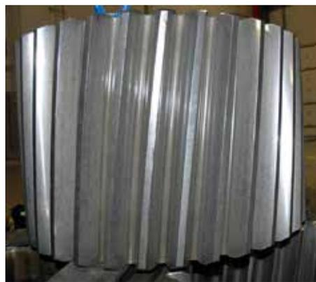
Figure 5: Three multi-megawatt class isotropic superfinished planets removed after seven years of operation.
