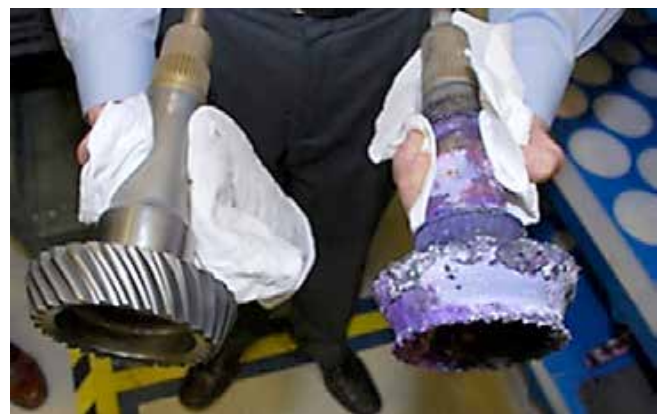
Figure 1: Left, an as-manufactured gear; right, the failed gear due to LOL gear (Aviation Investigation Report A09A0016).
