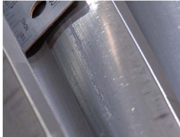
Figure 1a. Micropitting or gray staining on gear flanks
