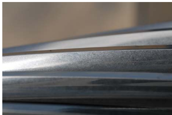
Figure 7b. Characteristic Isotropic Superfinish on the flanks of the intermediate gear assembly pictured above (photo courtesy of Moventas)
