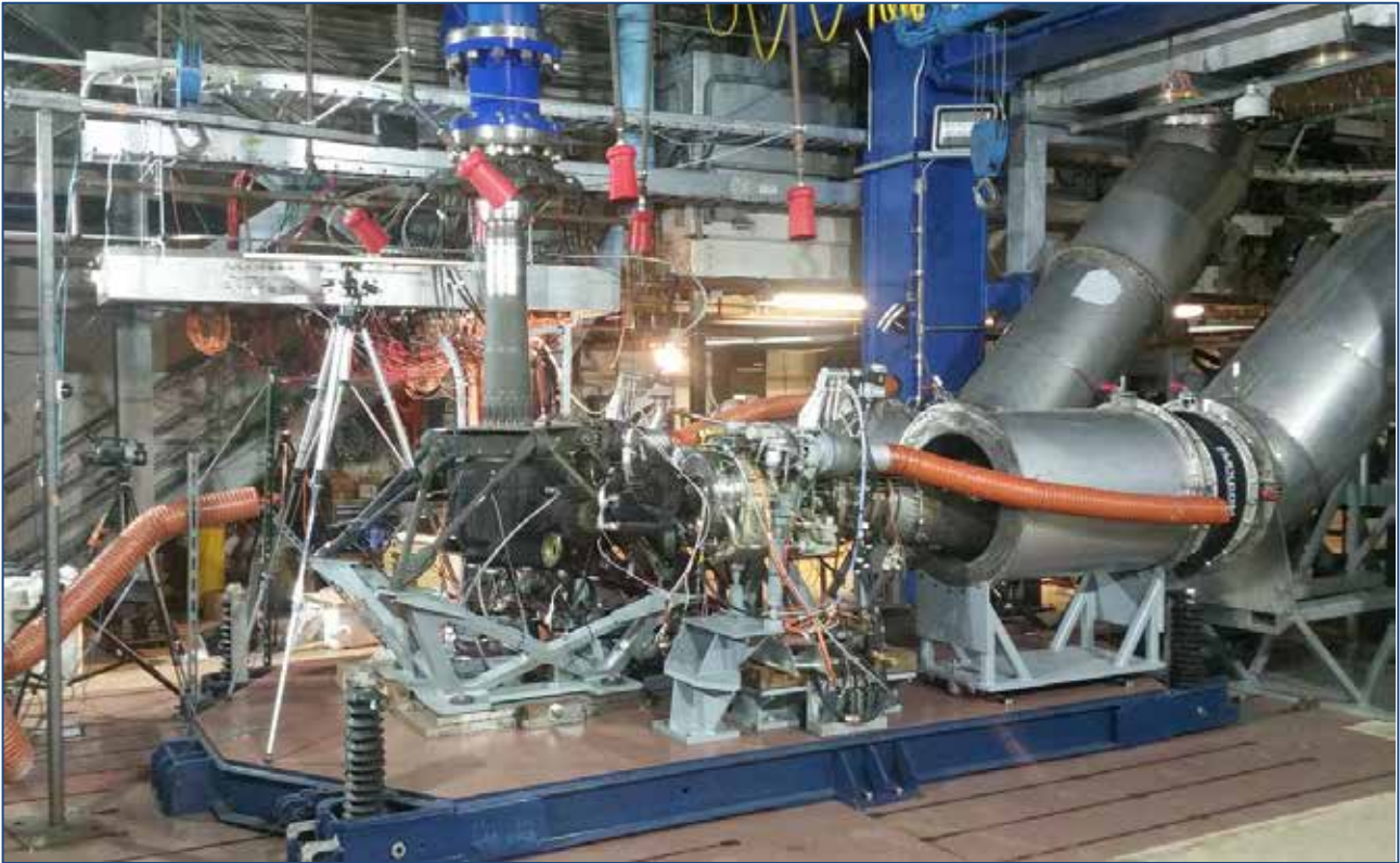
Figure 6. AH64 Apache Test Stand as configured for the LOL test.
