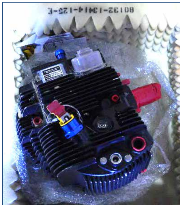
Figure 7. Front view of the Engine Nose Gearbox used in the LOL test.
