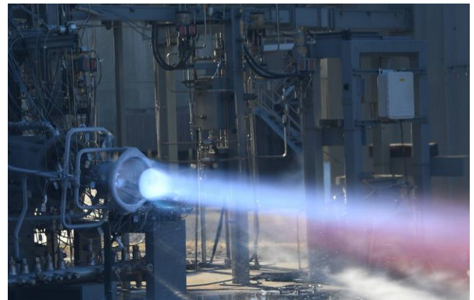
Figure 2: Additively manufactured (Laser Direct Energy Deposition) firing chamber and rocket nozzle processed by REM Optimized Finishing Technique survives 23+ hotfire tests (Source=NASA)
