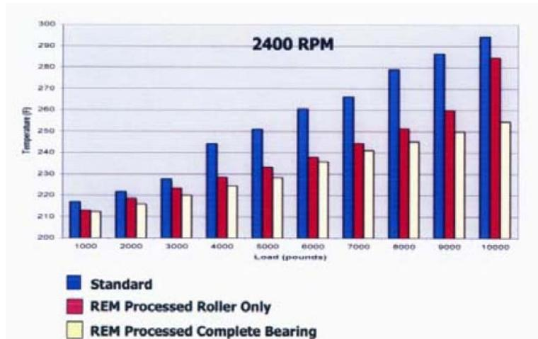
Figure 10 - Loading efficiency temperature test results for all three bearing sets. <sup>2,6,14</sup>
