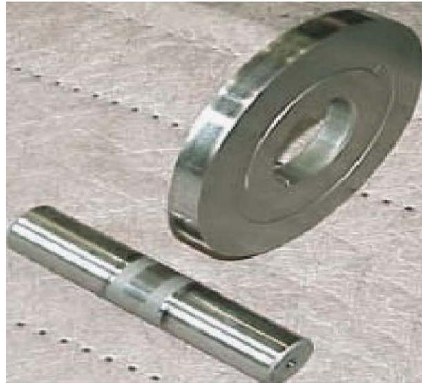
Figure 12 - A 1" diameter specimen pin at the lower left and a 5" loading roller at the upper right side of the photograph.<sup>2,7</sup>
