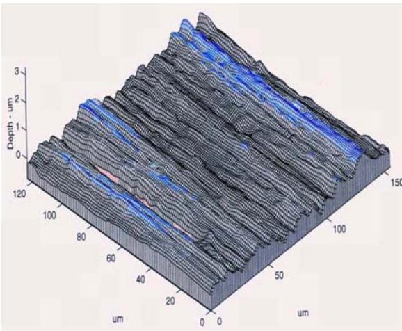
Figure 2 - A magnified view of a ground surface.<sup>1-3</sup> Note the unidirectional parallel rows of asperities corresponding to the final direction of the grinding operation.
