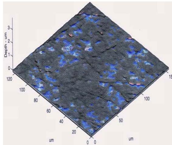
Figure 3 - A magnified view of an isotropically prepared surface.<sup>1-3</sup> Note, the parallel rows of asperity peaks as seen in Fig. 2 are non-existent and the final surface is smoother and random with no directional pattern.
