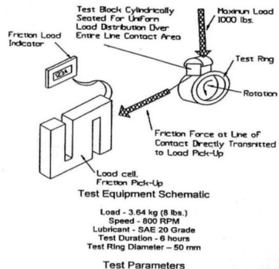
Figure 8 - A simplified schematic of the Block-on-Ring apparatus.<sup>3</sup>
