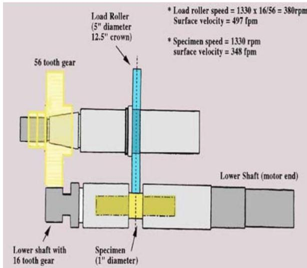
Figure 11 - Simplified schematic of the R/SCF Rolling / Sliding Contact Fatigue Test Rig.<sup>2,7</sup>
