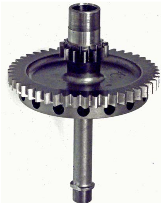
Figure 9. As received used/scrap carburized AISI 9310 gasifier train gearshaft
