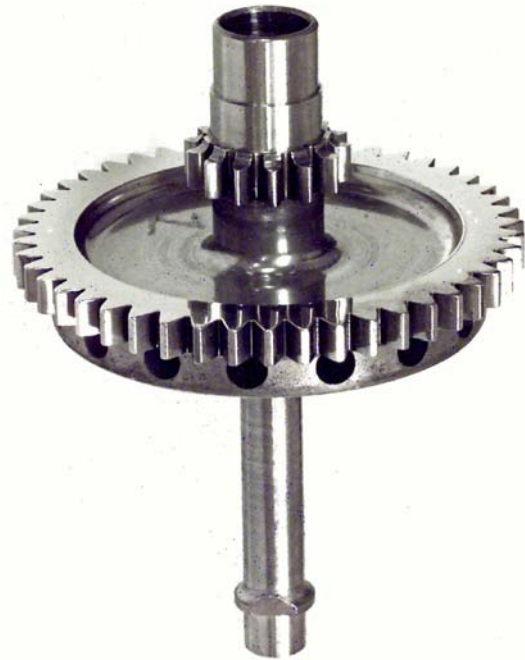
Figure 10. Superfinished used/scrap carburized AISI 9310 gasifier train gearshaft
